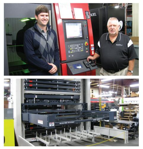
250 pieces (larger orders are 300 to 500 parts and the smallest orders range from two to 50 parts). Guzzo noted that the quality of the parts is also much improved. The tolerance of the old laser was  $\pm$  .012". With the new laser, he's seeing  $\pm$ .002" or .003". With the improved edge quality, Accrotool no longer needs to run secondary operations, improving throughput.
